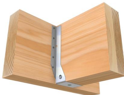
Double laminated joists to beam support, showing nail fix option. Screws can also be used refer to table for details.
