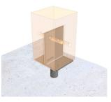
Drill through post using saddle holes. Ensure drill through holes are horizontally level and perpendicular to saddle.
