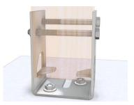
• Insert bolt through saddle and passing through timber post. A minimum of 2 x thread pitch should extend beyond the outward surface of the nut.
