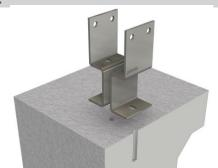
Drill two holes at marked location to required depth for selected hold-down bolt. Refer to bolt manufacturer guidelines for recommended pre-drill hole size and depth. Suggested minimum screw embedment depth 100mm or greater (section detail shown above).
